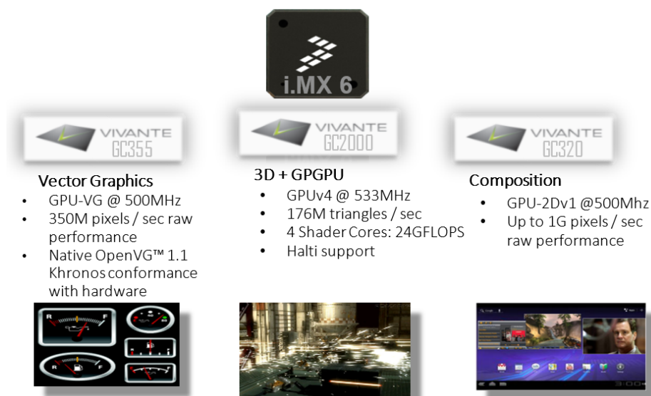
Figure 3. Freescale's i.MX6Q/D hosts three distinct GPUs
